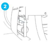
The torsion spring makes roller contact at a constant pressure on the handrail.
