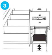
The rear roller and the handrail's rotational force generates power.
