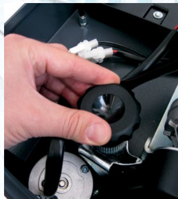
Main brush pressure adjustment
