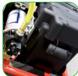
Pump relief safety valve
